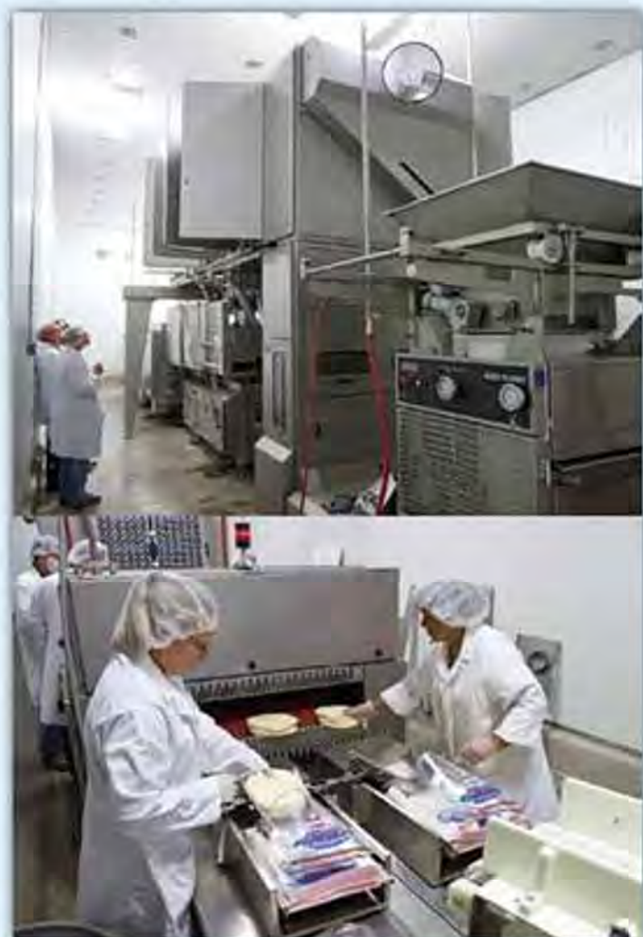
■ Requiring five Praters staff members to operate, the tortilla machine now produces two distinctly different products. The 'Mi Pueblo' recipe is a basic table tortilla but with superior quality. The second, 'Tejano Style,' represents an improvement over a home-style product.
