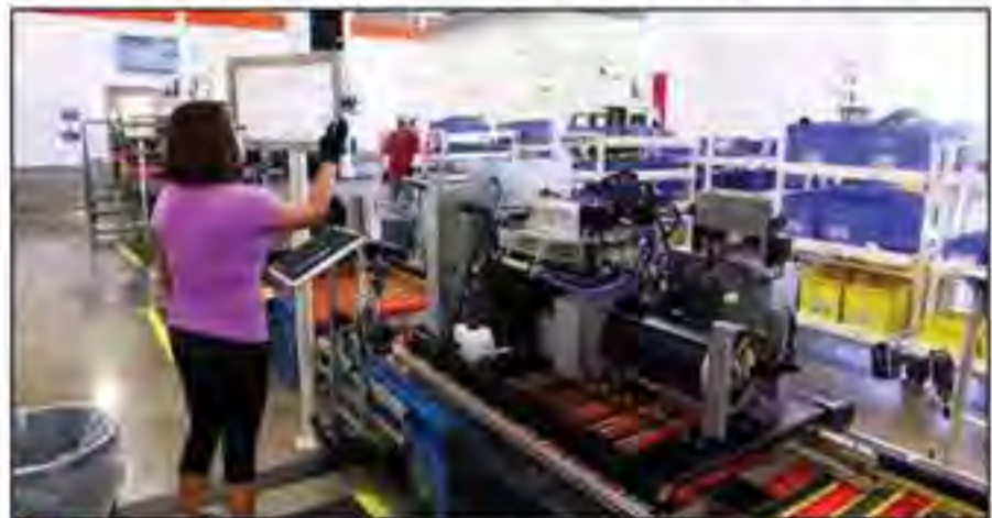
■ Operators now have real-time visual views on the line and can use touch-screen functionality to verify steps and quality control. They can also use their screen to signal to a supervisor if there's a problem or when the unit is ready to move to the next station; the station's signal light will change accordingly.
